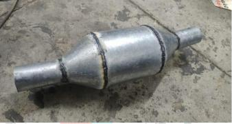
Figure 8 Catalytic ConverterTable 3 Specificationsof Catalytic ConverterCell Density500 cpsiMaterialMild SteelTotal Length375 mmCeramic SubstrateHoney Comb Structure
