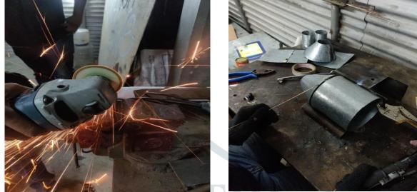
Figure 3 Cutting of sheet metal
