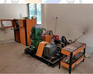
Figure 5. Diesel engine test rig
