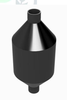
Figure 1 Two-dimensional design of Catalytic Converter
