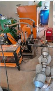
**Figure 9** Diesel engine exhaust having DPF,DOC and Catalytic converter
