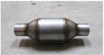
Figure 7 Diesel Oxidation Catalyst
