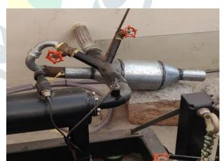
Figure 10 Diesel engine exhaust having Catalytic converter only
