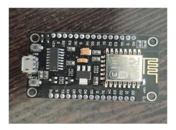
FIGURE 3. Node Microcontroller unit
