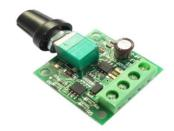
FIGURE 6. .Speed controlling unit
