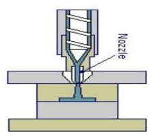
Clamp Mechanism: Clamping is used to keep the mould tightly closed under sufficient pressure to let the molten plastic fill in the cavity without leaking during the injection process.
