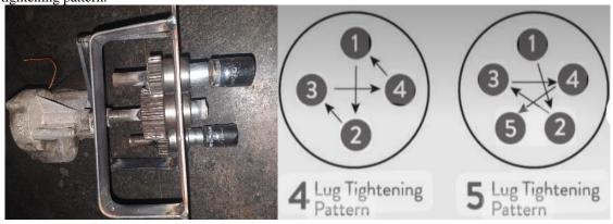
FIGURE 1: Multi-nut lightener and lug tightening pattern
