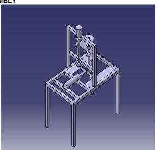
FIGURE 10. Isometric View of Fabricated Machine Vice
