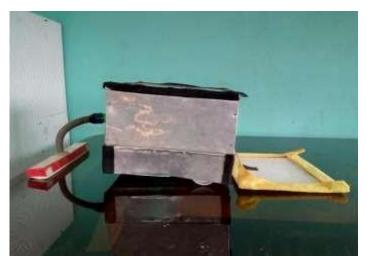
FIGURE 4. Semi-automatic floor cleaner
