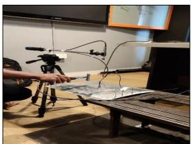
FIGURE 3: Experimental setup of Impact hammer method
