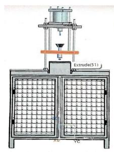
the insulation between piston rod and dies, a frame is used for the equal distribution of load on the material to be produced by using this machine. Molding compound is placed in an open and heated mold cavity. The mold is closed and the pressure is applied to force the material to fill up the entire mold cavity. The heat and pressure is maintained until the plastic material is cured. Once the material is cured it is removed from the mold for finishing.
