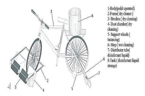
FIGURE 2. Manually operated floor cleaning machine
