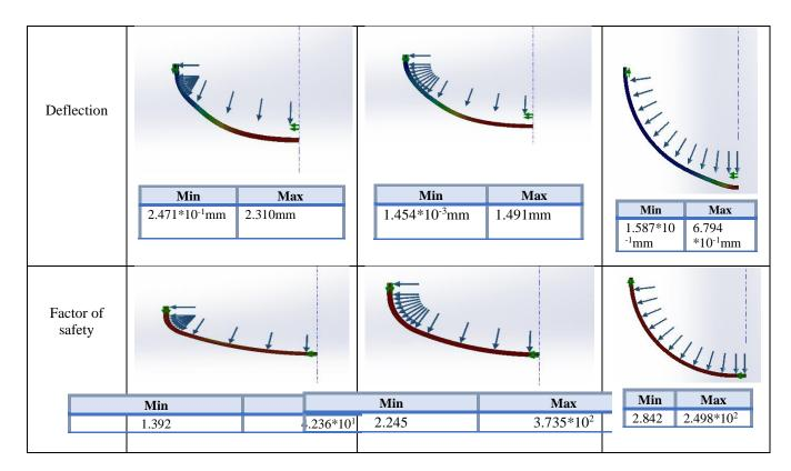
Chemicals, fuels, and gases exert a maximum internal pressure of 2MPa and the thickness of the dished ends is calculated for the same internal pressure. The analysis for the dished ends is made for the same pressure. The analysis is done for Von-mises stress, deflection, and factor of safety. The result of the analysis declared the modelled parts as safe.
