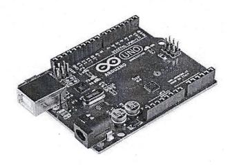
microcontroller. ATmega328P has 14 digital input/output pins. It has 6 analog input/output/pins. It can be programmed with the help of Arduino Integrated
