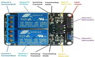
**FIGURE 3:** 2 Channel Relay Module [13]
