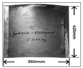
FIGURE2: Fabricated shell structures.
