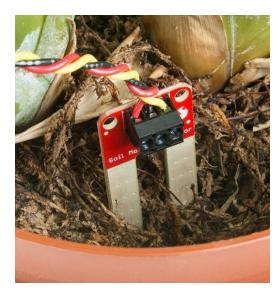
FIGURE 1. Soil moisture sensor
