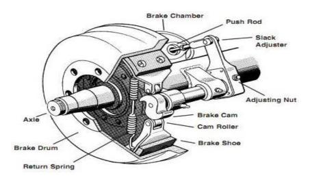
Fig 2.2, Air brake system.
