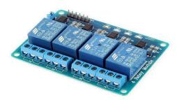
FIGURE 5. Relay switch
