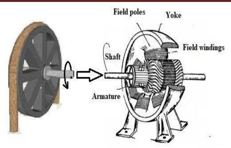
**FIGURE 4.** Output of pulley connected to alternator
