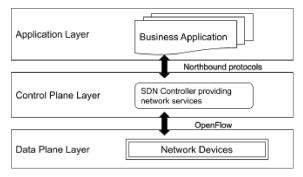
Fig. 1. Three-layered architecture of SDN
