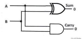
Figure 1: Half Adder circuit
