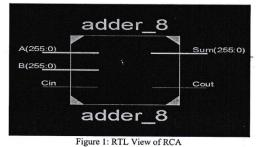
Logical Expression for SUM: = A' B' C-IN + A' B C-IN' + A B' C-IN' + A B C-IN = C-IN (A'B' + AB) + C-IN' (A'B + AB')
