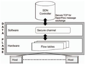
Fig. 2. OpenFlow communication between SDN switch and controller
