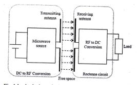
Fig.1 basic design of wireless power transmission
