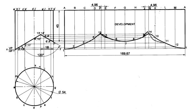
**Problem 33** A vertical cylinder of base diameter 50mm and axis length 60mm is cut by a two planes which are perpendicular to VP and inclined at 45° to HP and passing through either side the centre point of the top face. Draw the development of the lateral surface of the cylinder.
