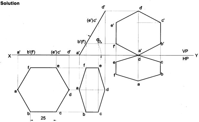
**Problem 38** A hexagonal lamina of sides 30mm is resting on HP with one of its corners in VP and its surface inclined at an angle of 30° with VP. The diagonal passing through that corner which is in VP is inclined at 45° to HP. Draw the projections of the lamina.
