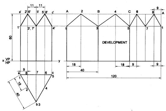
**Problem 2** A square prism of base side 30 mm and axis length 60 mm is resting on HP on its base with all the vertical faces being equally inclined to VP. It is cut by an inclined plane 60° to HP and perpendicular to VP and is passing through a point on the axis at a distance 50 mm from the base. Draw the development of the lower portion of the prism.
