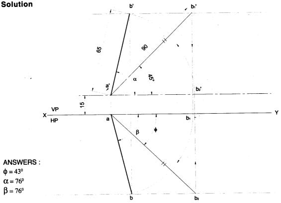
**Problem 12** The distance between the end projectors through the end points of a line AB is 60 mm. The end A is 10 mm above HP and 15 mm infront of VP. The end B is 35 mm infront of VP. The line AB appears 70 mm long in the front view. Complete the projections. Find the true length of the line and its inclinations with HP and VP.
