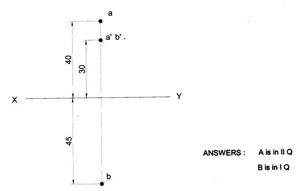
**Problem 5** A point 'A' is 30 mm in front of VP and 40mm above HP. Another point B is 20 mm behind VP & 35 mm below HP. The horizontal distance between the points measured parallel to XY line is 60 mm . Draw the three projections of the points. Join their front and top views.
