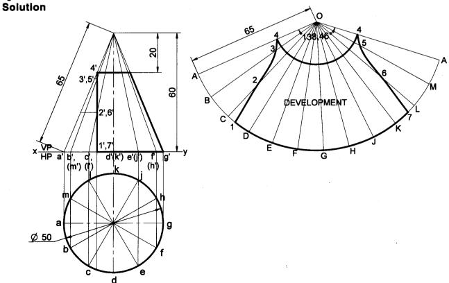
**Problem 49** A funnel is to be made of sheet metal. The funnel tapers from 40 mm to 20 mm diameter to a height of 20 mm and from 20 mm to 15 mm diameter, for the next 20 mm height. The bottom of the funnel is beveled off to a plane inclined at 45° to the axis. Draw the development of the funnel.
