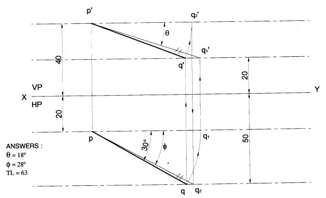
**Problem 21** The top view of a line PQ is 70 mm and front view is 60 mm long. The end Q is nearer to both HP and VP than the end P and is 15 above HP and 20 mm infront of VP. Draw the projections of the line if the distance between projectors is 50 mm.
