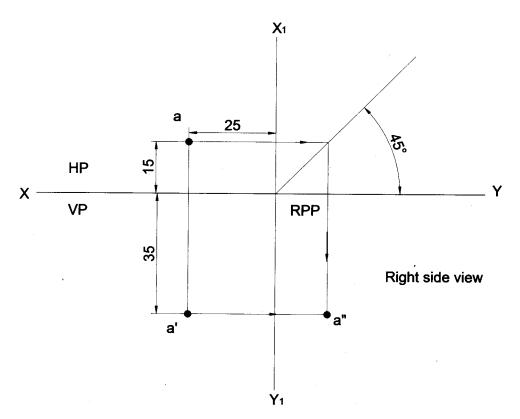
**Problem 48** A point P is 15 mm above HP & 25 mm in front of VP. Another point Q is 25 mm behind VP and 40 mm below HP. Draw their projections when the distance between their projectors parallel to XY line is zero mm. Add the right side view only to point Q.
