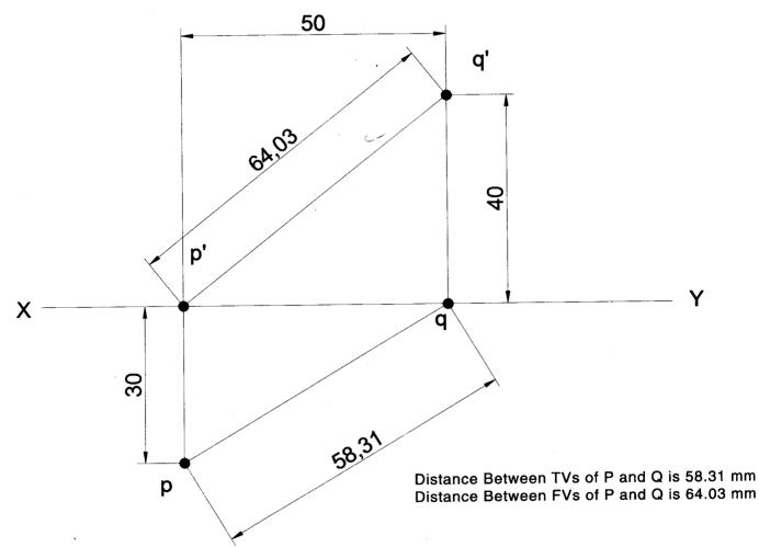
**Problem 39** Draw the projections of a point A lying 30 mm above HP and in first quadrant, if its shortest distance from the line of intersection of HP and VP is 50 mm. Also find the distance of the point from VP. **Solution**
