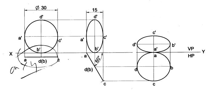
**Problem 50** A circular lamina of 30mm diameter rests on VP such that one of its diameters is inclined at 30° to VP and 45° to HP. Draw its top and front views in this position. **Solution**
