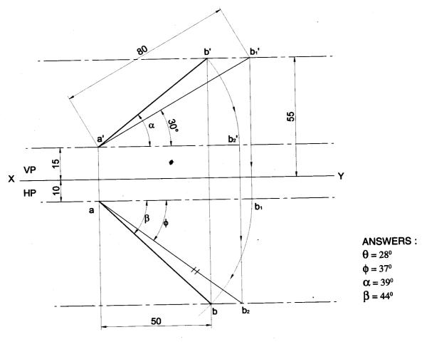
**Problem 46** The end A of a line AB is in HP and 25mm in front of VP. The end B is 10 mm in front of VP and 50mm above HP. The distance between the end projectors when measured parallel to the line of intersection of HP & VP is 80 mm. Draw the projections of the line AB and determine its true length and true inclinations with HP & VP. **Solution**
