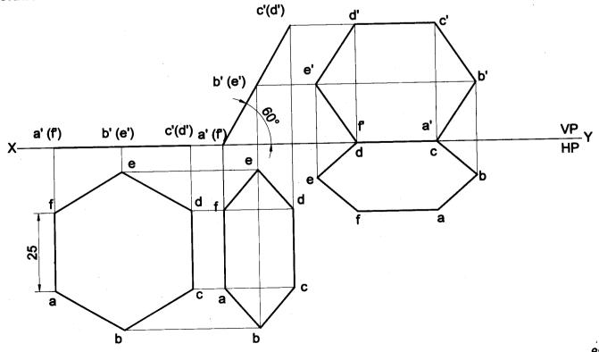
**Problem 37** A regular hexagonal lamina of side 25mm is lying in such a way that one of its corners on HP while the corner opposite to the corner on which it rests is on VP. If the lamina makes 60° to HP, Draw the projections of the lamina.
