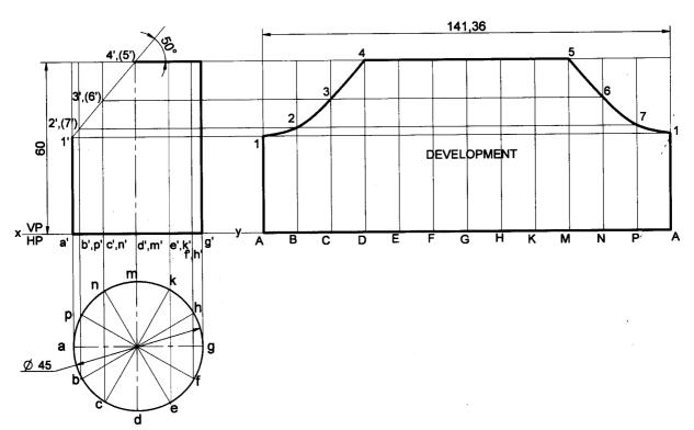
**Problem 32** Following figure shows the front view of a model of a steel chimney of diameter 60mm made from a flat thin sheet metal fitted over an inclined plane roof. Develop the portion of the chimney. **Solution**
