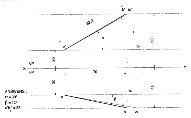
**Problem 4** A line AB has its end A 20 mm above the HP and 15 mm infront of the VP. The other end B is 60 mm above the HP. The distance between end projectors is 70 mm. draw its projections. Determine the apparent lengths and true inclinations.
