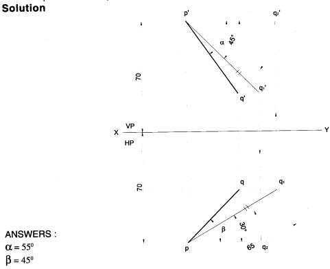
**Problem 20** A point P is 40 mm above HP and 20 mm infront of VP another point Q is 20 mm above HP and 50 mm infront of VP. The top view of line PQ is inclined at 30° to XY. Draw the projections. **Solution**
