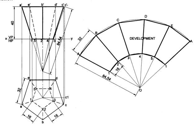
**Problem 24** A regular pentagonal pyramid of side of base 35mm and altitude 65mm has its base on HP with a side of base perpendicular to VP. The pyramid is cut by a section plane which is perpendicular to the VP and inclined at 30° to HP. The cutting plane meets the axis of the pyramid at a point 30mm below the vertex. Obtain the development of the remaining part of the pyramid.
