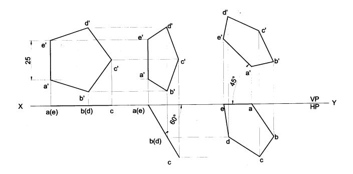
**Problem 30** A pentagonal lamina having edges 25mm is placed on one of its corners on VP such that the surface makes an angle 30° with VP and perpendicular bisector of the edge passing through the corner on which the lamina rests appears to be inclined at 30° to HP. Draw the top and front views of the lamina. **Solution**
