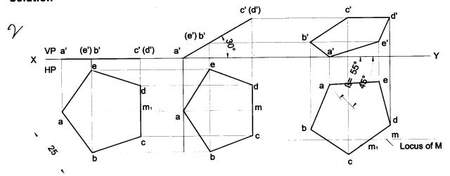
**Problem 24** A pentagonal lamina of sides 25mm is having a side both on HP and VP. The corner opposite to the side on which it rests is 15mm above HP. Draw the top and front views of the lamina.
