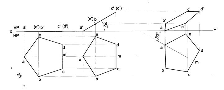
**Problem 28** A regular pentagonal lamina of 25mm side is resting on one of its sides on HP while the corner opposite to this side touches VP. If the lamina makes an angle of 60° with HP and 30° with VP, draw the projections of the lamina.
