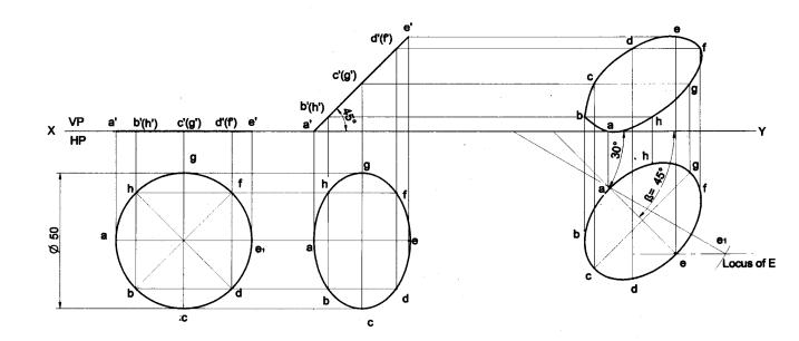
**Problem 49** A circular lamina inclined to the VP appears in the front view as an ellipse of major axis 30mm and minor axis 15mm. The major axis is parallel to both HP and VP. One end of the minor axis is in both the HP and VP. Draw the projections of the lamina and determine the inclination of the lamina with the VP. **Solution**
