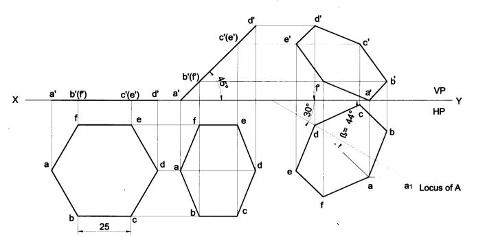
**Problem 42** A hexagonal lamina of sides 25mm rests on one of its corners on HP. The lamina makes 45° to HP and the diagonal passing through the corner on which it rests appears to be inclined at 30° to VP. Draw its projections. **Solution**
