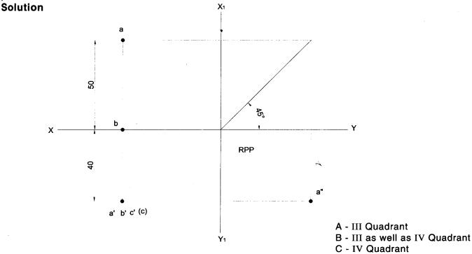
**Problem 31**A point A is on HP and 35 mm in front of VP. Another Point B is on VP and below HP. The line Joining their front views makes an angle of 30 deg to XY line while the line joining their top views makes an angle 45 deg with XY line. Find the distance of the point B from HP.
