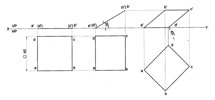
**Problem 9** A square plate of 30mm sides rests on HP such that one of the diagonals is inclined at 30°to HP and 45° to VP. Draw its projections.
