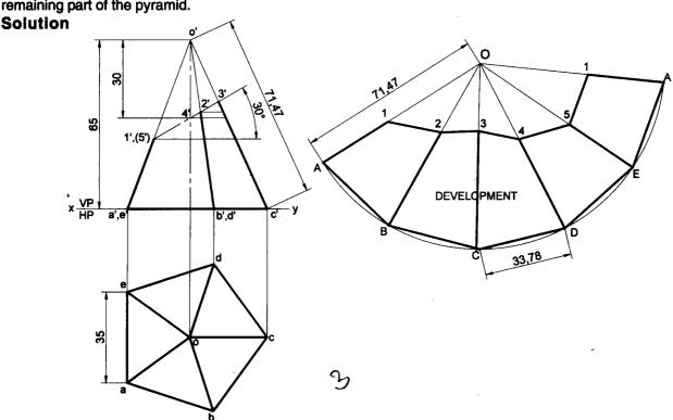
**Problem 25** A pentagonal pyramid, 30mm sides, with a side of base perpendicular to VP. Draw the development of the lateral surfaces of the retained portion of the pyramid shown by the dark lines in the following figure.
