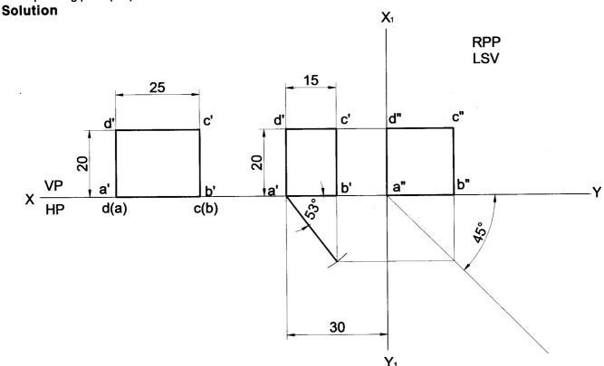
**Problem 16** The front view of a rectangular lamina of sides 30mm x 20mm is square of 20mm sides. Draw the projections and determine the inclinations of the surface of the lamina with HP and VP. **Solution**
