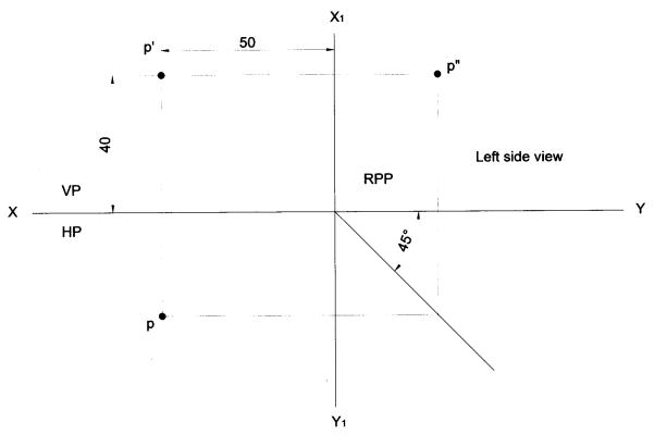
**Problem 16** The point P is 45 mm above HP, 60 mm behind VP and 30 mm from RPP. Draw the three principles view of the point. Also state the quadrant in which it lies. **Solution**
