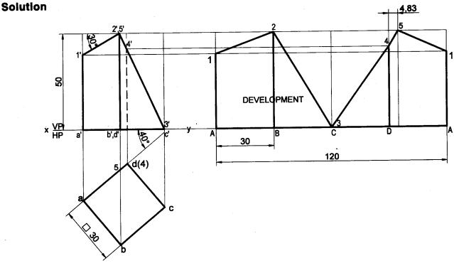
**Problem 5** A cube of side 40mm is resting on HP with its base on HP such that one of its vertical faces is inclined at 30° to the VP. It is cut by a section plane perpendicular to VP, inclined to HP at an angle 45° and passes through the midpoint of the axis. Draw the development of the lower lateral surface of the cube. **Solution**
