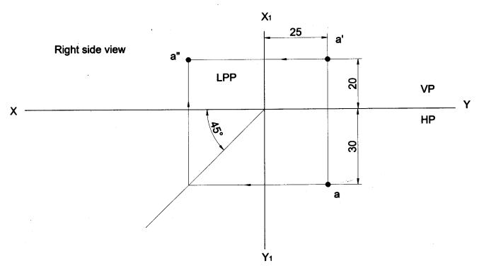
**Problem 19** A point is 40 mm behind VP, 15 mm above HP and 25 mm in front / behind / from LPP .Draw its projections and name the side view.
