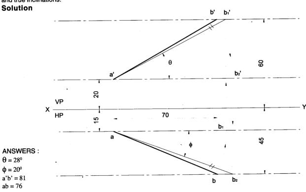
Problem 5 The top view PQ of a straight line is 70 mm and makes an angle of 60° with XY line. The end Q is 10 mm infront of VP and 30 mm above the HP. The difference between the distances of P and Q above the HP is 45 mm. draw the projections. Determine its true length and true inclinations with HP and VP. Solution
