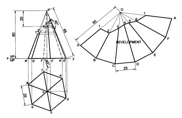
**Problem 28** A hexagonal pyramid of sides 35mm and altitude 65mm is resting on HP on its base with two of the base sides perpendicular to VP. The pyramid is cut by a plane inclined at 30° to HP and perpendicular to VP and is intersecting the axis at 30mm above the base. Draw the development of the remaining portion of the pyramid. **Solution**
