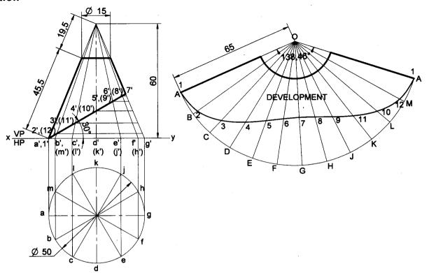
**Problem 46** A cone of base diameter 50mm and height 60mm is resting with its base on HP. It is cut, as shown in the following front view of which is as shown in figure. Draw the development of the lateral surface of it. **Solution**
