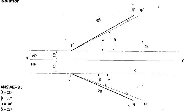
**Problem 7** A line has its end A 10 mm above HP and 15 mm infront of VP. The end B is 55 mm above HP and line is inclined at 30° to HP and 35° to VP. The distance between the end projectors is 50 mm. draw the projections of the line. Determine the true length of the line and its inclination with VP.
