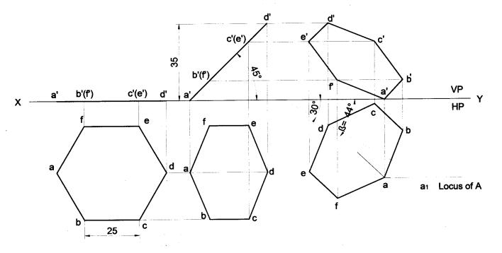
**Problem 46** Draw the projections of a circular plate of negligible thickness of 50mm diameter resting on HP on a point A on the circumference, with its plane inclined at 45° to HP and the top view of the diameter passing through the resting point makes 60° with VP.
