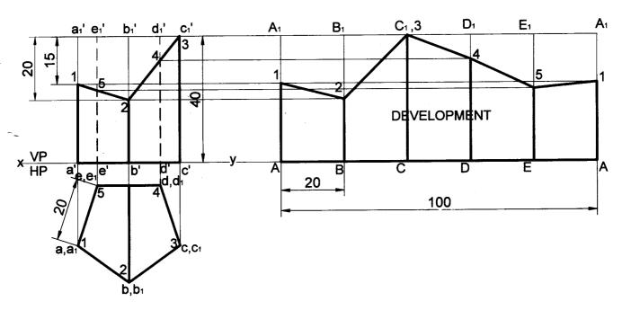
**Problem 15** A hexagonal prism of base side 20mm and height 50mm is resting on HP on its base, such that one of its base edge is parallel to VP. The prism is cut in this position as shown in the following front view. Draw the development of the lateral surface of the prism.
