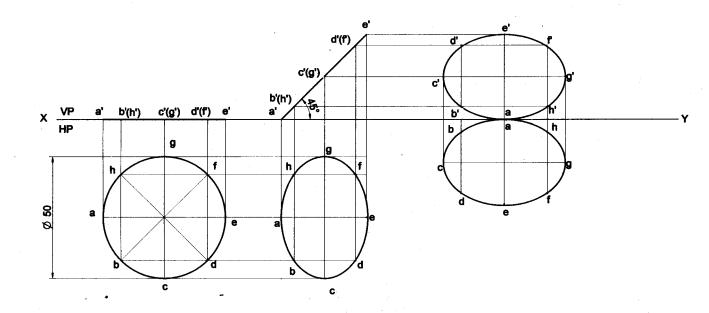
**Problem 48** A circular lamina of 50mm diameter rests on HP such that one of its diameters is inclined at 30° to VP and 45° to HP. Draw its top and front views in this position. **Solution**
