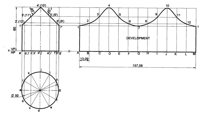
**Problem 34** A pipe made of using a half tubular (circular) with a half square in shape is cut as shown in the following figure. Draw the development of the lateral surface of the object. **Solution**
