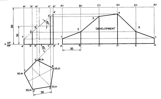
**Problem 14** A pentagonal prism of base sides 20mm and height 40mm is resting with its base on HP and base edge parallel to the VP. The prism is cut as shown in the following front view. Draw the development of the lateral surface of the prism.
