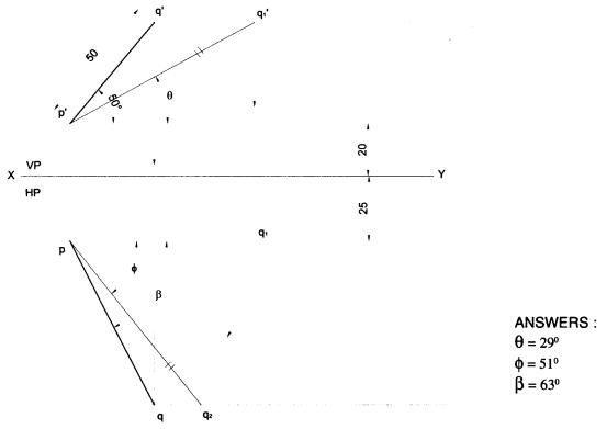
**Problem 30** Draw the projections of a line AB 100 mm long inclined at  $45^0$  to VP and  $30^0$  to HP. One end of the line is 20 mm above the HP and in the VP. Also determine the apparent length and inclinations. **Solution**
