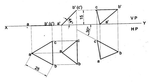
**Problem 6** A 30°-60° setsquare of 60mm longest side is so kept such that the longest side is in HP, making an angle of 30° with VP. The set square itself is inclined at 45° to HP. Draw the projections of the setsquare. **Solution**
