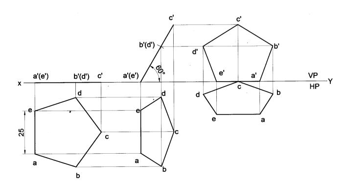
**Problem 29** A pentagonal lamina of edges 25mm is resting on VP with one of its sides such that the surface makes an angle of 60° with VP. The edge on which it rests is inclined at 45° to HP. Draw its projections. **Solution**
