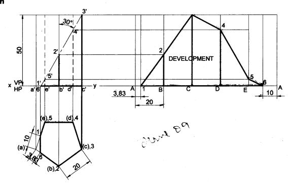
**Problem 11** A regular pentagonal prism of height 60mm and base edge 30mm rests with its base on HP. The vertical face closest to VP is 30° to it. Draw the development of the truncated prism with its truncated surface inclined at 60° to its axis and bisecting it.
