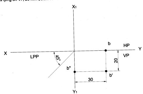
**Problem 24** A point A is 20 mm above HP & 25 mm in front of VP. Another point B is 25 mm behind VP and 40 mm below HP. Draw their projections when the distance between their projectors parallel to XY line is zero mm. Add the right side view only to point B.
