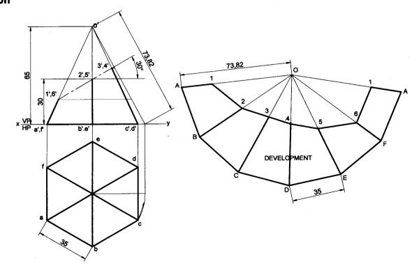
**Problem 29** A hexagonal pyramid 25 mm side of base and axis 65 mm long is resting on its base on HP with one of the edges of the base parallel to VP. It is cut by a vertical section plane at a distance of 8 mm from the axis towards right side. Develop the lateral surface of the left part of the pyramid.
