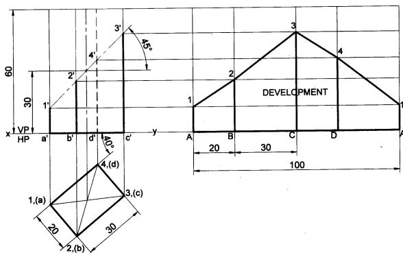
**Problem 9** A rectangular prism of base size 25mm×40mm and axis length 65mm is resting on HP on its base with the lenger side of base inclined at 30° to VP. It is cut by a plane inclined at 40° to HP and perpendicular to VP and passes through the extreme left comer of base. Draw the development of the lateral surface of the remaining portion of the prism.
