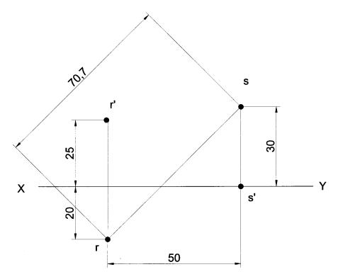
**Problem 13** A point M is on HP & 30 mm in front of VP. Another point N is 20 mm below HP and 20 mm in front of VP. The distance between their projectors measured parallel to XY line is 50 mm. Find the distance between front views of the points M & N.
