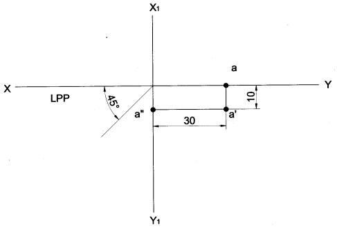
Choice 1: Treating the point is in III Quadrant, it is left side view Choice 2: Treating the point is in IV Quadrant, it is right side view
