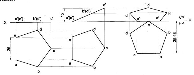
**Problem 23** A pentagonal lamina having edges 25mm is placed on one of its corners on HP such that the perpendicular bisector of the edge passing through the corner on which the lamina rests is inclined at 30° to HP and 45° VP. Draw the top and front views of the lamina.
