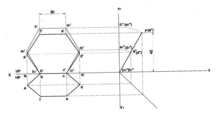
**Problem 36** A regular hexagonal lamina of sides 25mm is lying in such a way that one of its sides on HP while the side opposite to the side on which it rests is on VP. If the lamina makes 60° to HP, Draw the projections of the lamina. **Solution**
