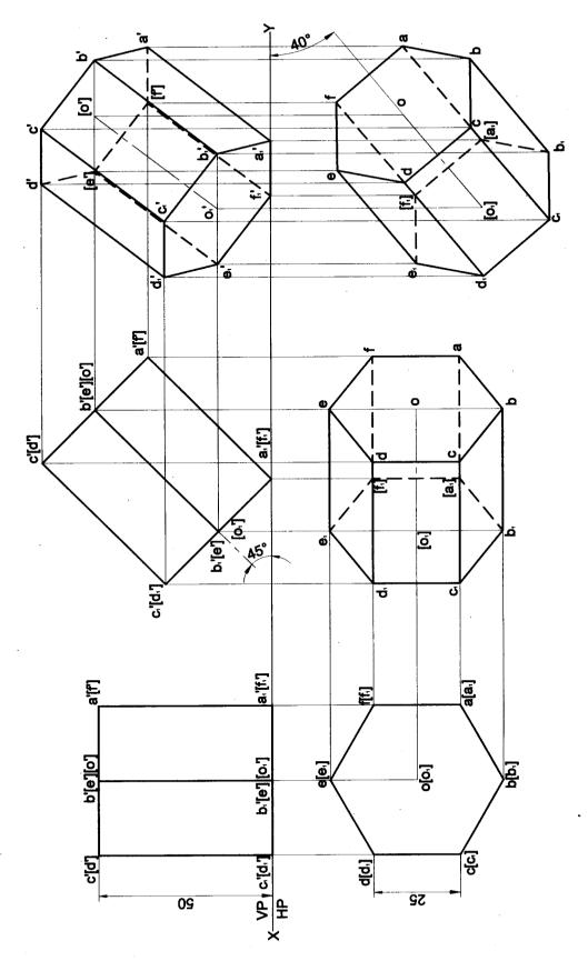
**Problem 10** A hexagonal prism 25 mm sides of base and 50 mm axis length rests on HP on one of its edges of the base. Draw the projections of the prism when the axis is inclined to HP at 45° and VP at 30°. **Solution**
