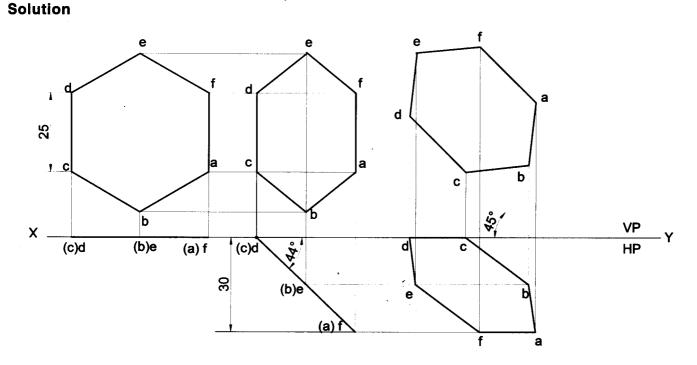
**Problem 45** A hexagonal lamina of sides 25mm rests on one of its corners on HP. The corner opposite to the corner on which it rests is 35mm above HP and the diagonal passing through the corner on which it rests is inclined at 30° to VP. Draw its projections. Find the inclination of the surface with HP.
