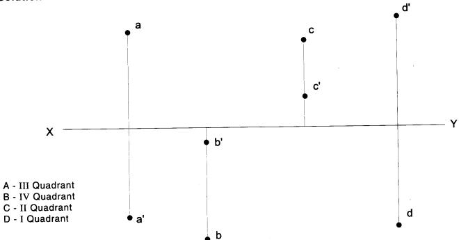
**Problem 4** A point 30mm above XY line is the front view of two points A&B .The top view of A is 40 mm behind VP & The top view of B is 45 mmin front of VP. Draw The projections of the points & state the quadrants in which the points are situated.
