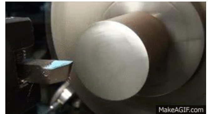
(a) Front view of facing operation
