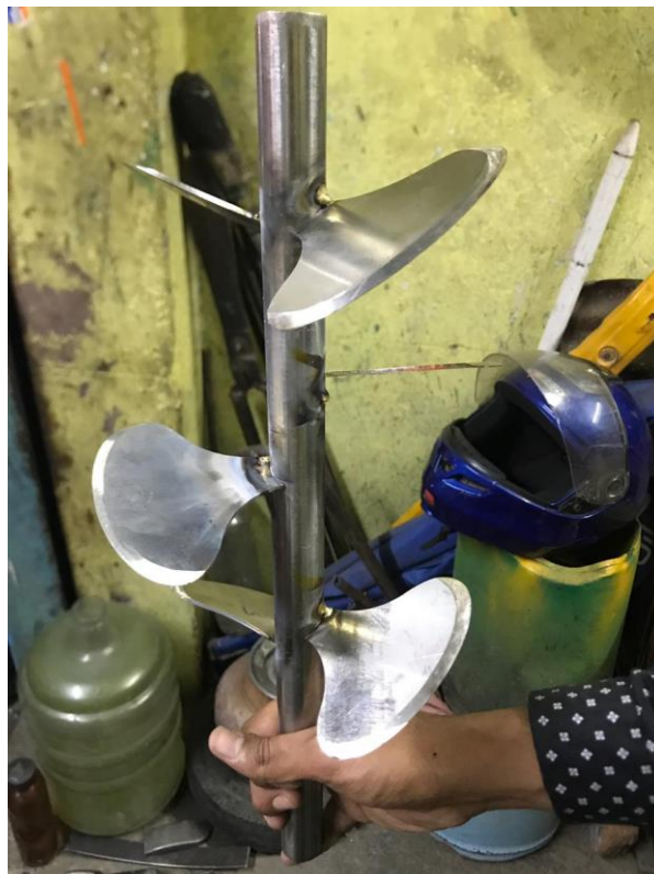
Fig 5.7 Construction of shredder blade
