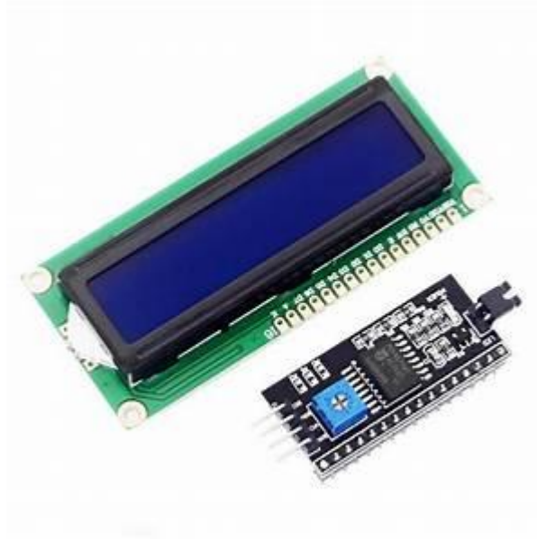
Fig. 6.1.8 Adafruit LCD with I2C module
