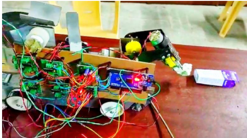
Fig-1: Once the sensor detects the waste, robot stops and arm picks the waste.
